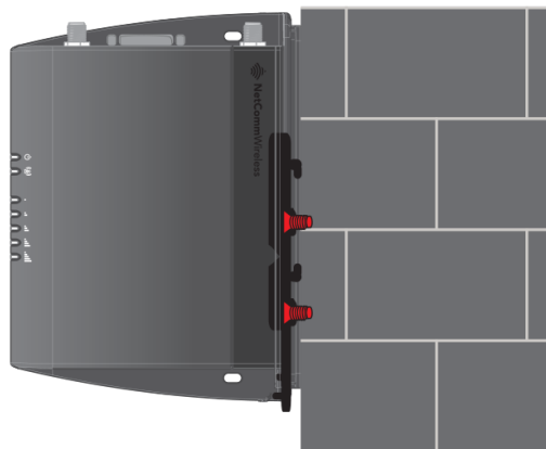
Figure 10 – Wall mount - Mounted via DIN rail bracket
