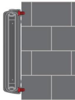
Figure 4 - Wall mount - Flat against the wall
