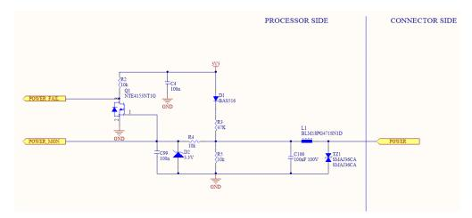
The Power detection or Ignition input will detect the presence of three states from the connector side (outside world). It will detect three states, those being High, Low and Unconnected (floating).
