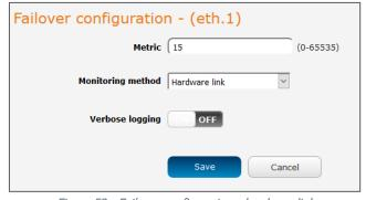
Figure 59 – Failover configuration – hardware link
