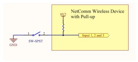
The following input detects an input going high. The turn on/off threshold can be set in the software.
