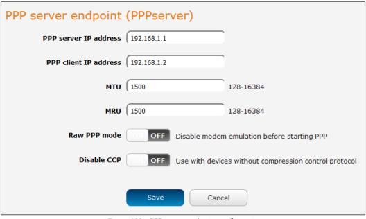
Figure 102 – PPP server endpoint configuration
