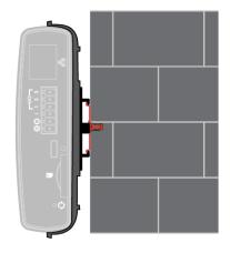
Figure 9 – Wall mount with DIN rail mount adapter
