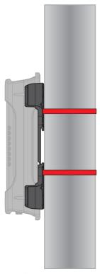
Figure 12 – Pole mount using DIN rail bracket
