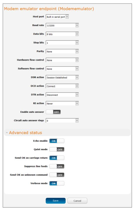
Figure 101 – Modem emulator endpoint configuration
