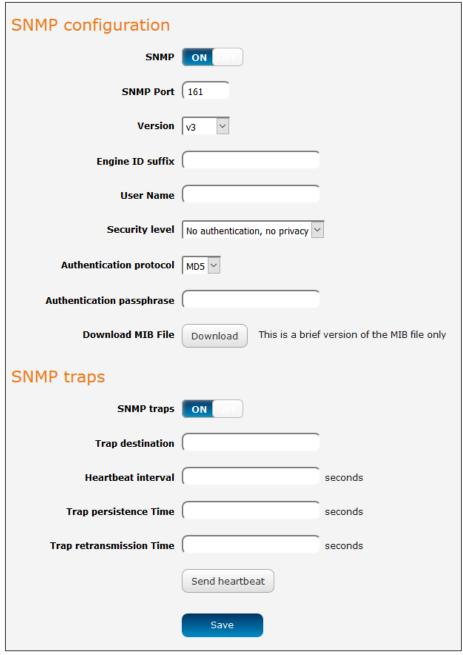
Figure 109 – SNMP configuration
