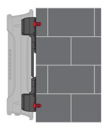
Figure 10 – Wall mounted via DIN rail bracket
