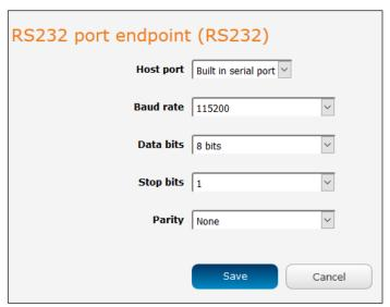
Figure 100 – RS232 / RS485 / RS422 port configuration options
