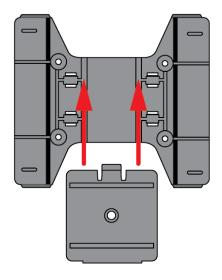
Figure 8 - Horizontal DIN rail mounting adapter
