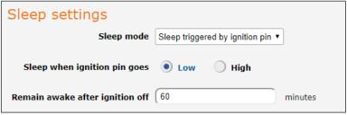
Figure 156 – Sleep triggered by ignition pin
