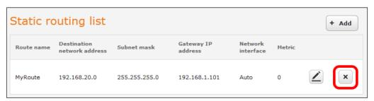
Figure 64 – Deleting a static route
