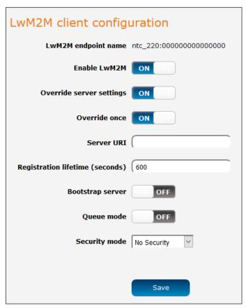
Figure 113 – LwM2M client configuration
