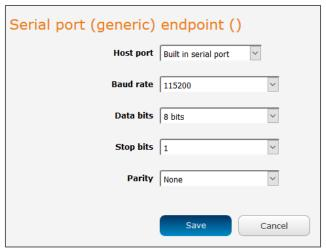
Figure 93 – Serial port (generic) endpoint configuration
