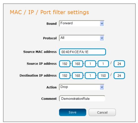
Figure 74 – MAC / IP / Port filtering settings
