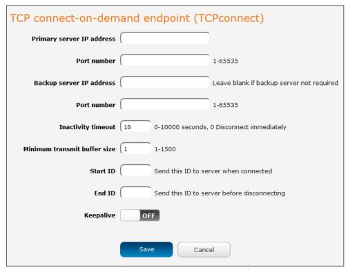
Figure 103 – TCP connect-on-demand endpoint configuration
