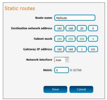
Figure 62 – Adding a static route
