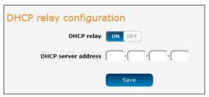
Figure 50 - DHCP relay configuration
