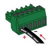
Figure 14 - Terminal block wiring diagram
