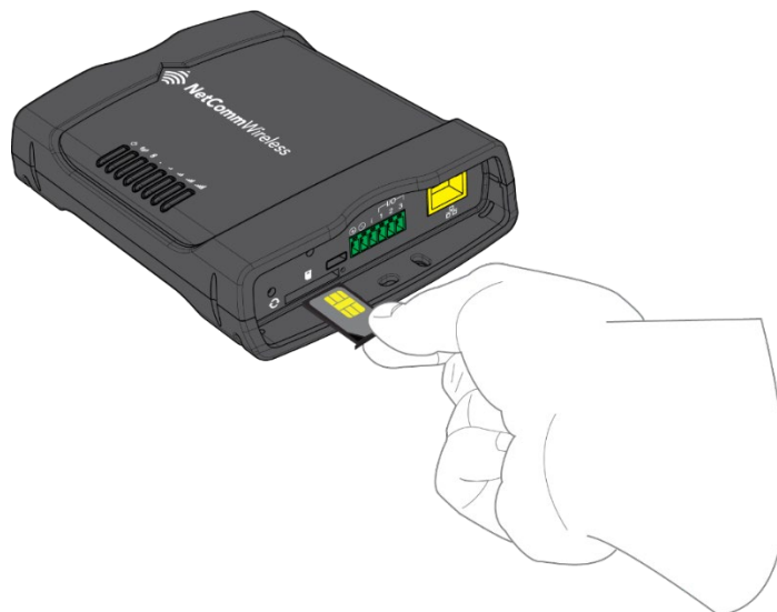
Figure 17 – Inserting the SIM card
