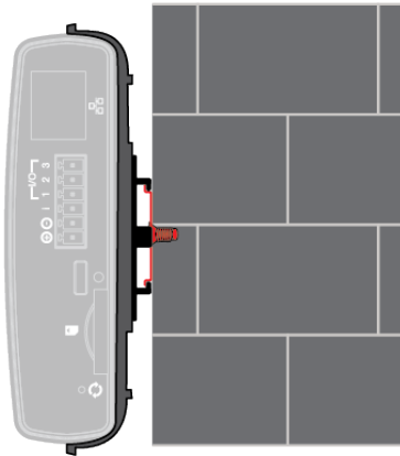
Figure 9 – Wall mount with DIN rail mount adapter
