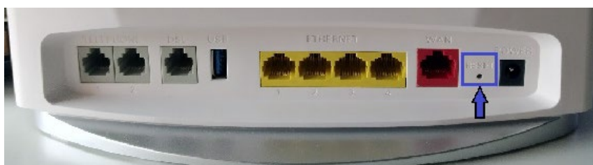
Back panel of Gateway showing Reset pinhole
