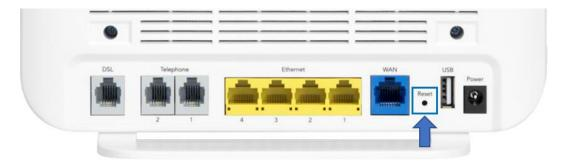
Back panel of NF18ACV showing Reset pinhole
