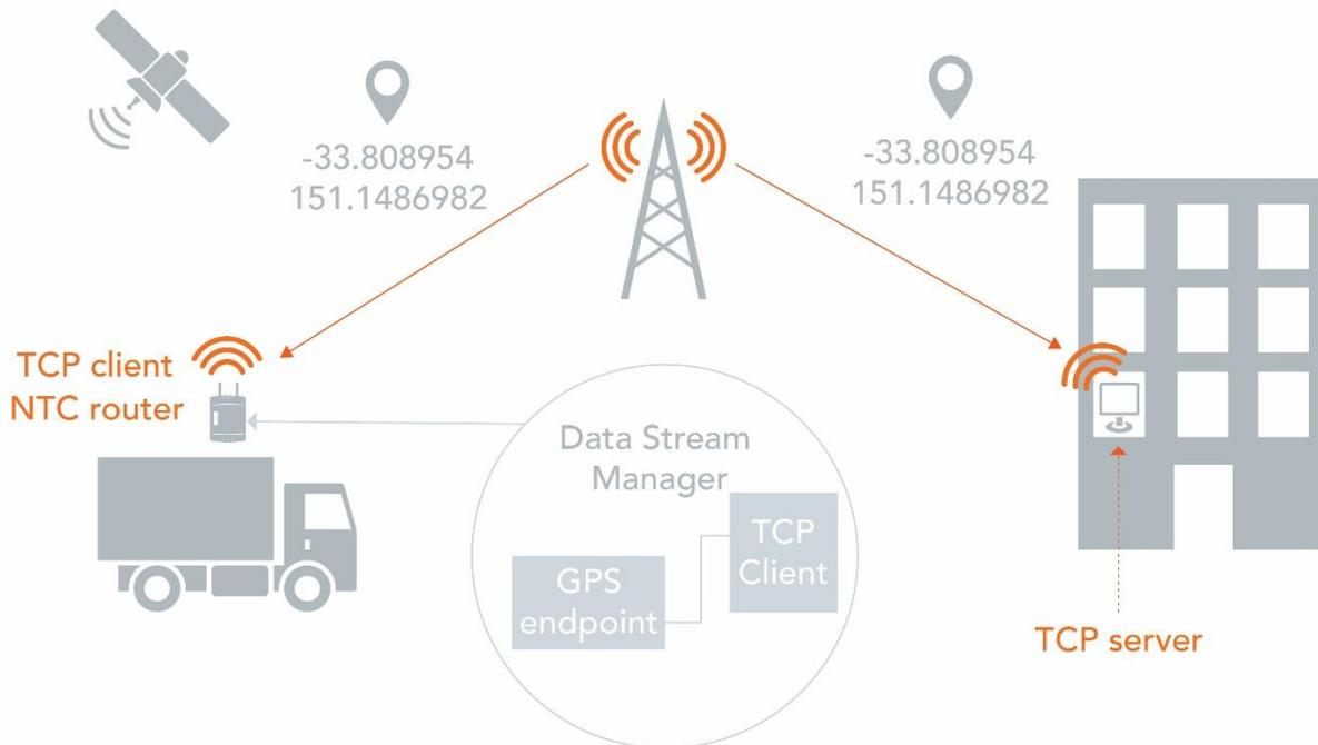
The GPS data is sent as raw (NMEA format) data and traverses through a TCP client (endpoint B) on the router to a remote TCP server. The GPS data can then be manipulated on the receiving end to plot the location on a map.
