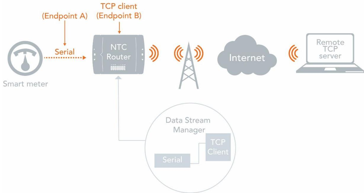
The data received on the serial port (endpoint A) is converted to IP data and traverses through a TCP client (endpoint B) on the router to a remote TCP server.
