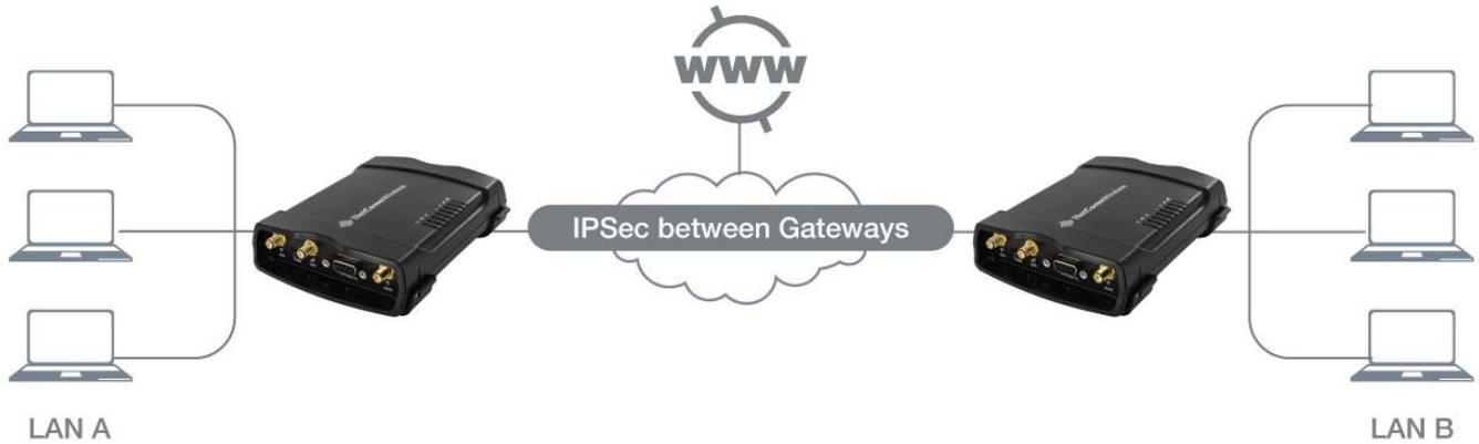
Figure 12 - IPsec Site to Site VPN tunnel between two NetComm Wireless routers using RSA key mode network diagram and policy planning
