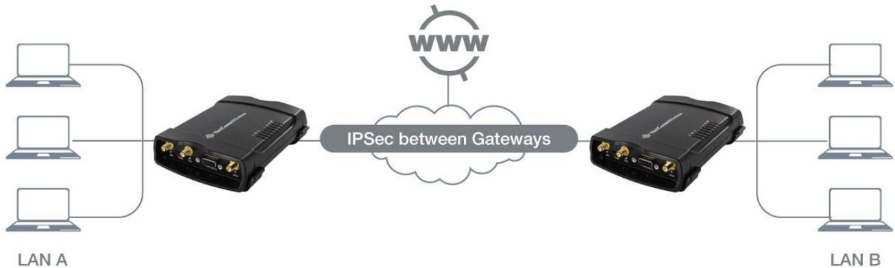
Figure 17 - IPsec Site to Site VPN tunnel between two NetComm Wireless routers using Digital Certificate mode network diagram and policy planning
