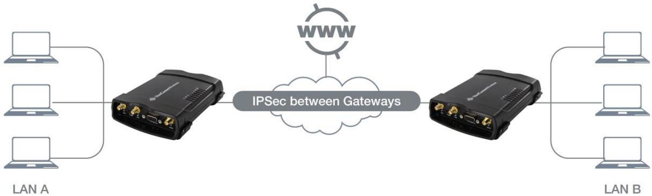
Figure 7 - IPsec Site to Site VPN tunnel between two NetComm Wireless routers network diagram and policy planning
