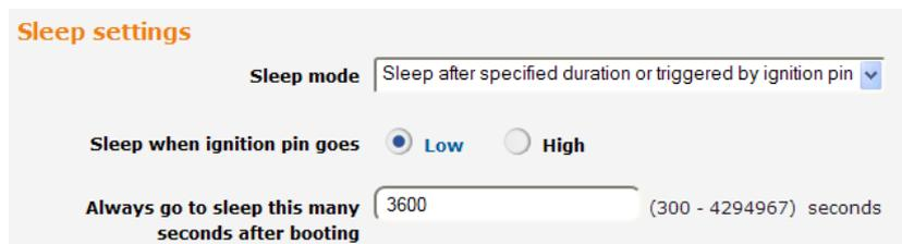
The screenshot shows the 'Sleep settings' section with the 'Sleep mode' dropdown menu set to 'Sleep after specified duration or triggered by ignition pin'. Below the dropdown are two radio buttons labeled 'Sleep when ignition pin goes' with options 'Low' (selected) and 'High'. Below that is a text input field labeled 'Always go to sleep this many seconds after booting' with the value '3600' and a range '(300 - 4294967) seconds'.
