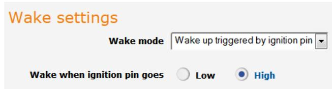
The screenshot shows the 'Wake settings' section. The 'Wake mode' dropdown menu is set to 'Wake up triggered by ignition pin'. Below it, the 'Wake when ignition pin goes' section has two radio buttons: 'Low' (unselected) and 'High' (selected).
