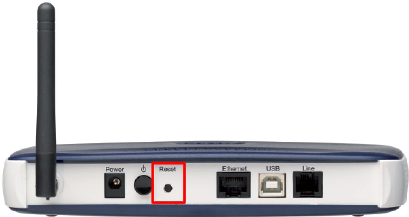
2. Use a thin object such as a paperclip to depress and hold in the reset button at the back of the modem for 20 seconds. During this time the modem lights will flicker in a pattern to show the reset is underway.
